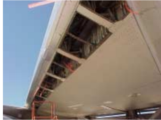
Figure 2-4: L1011 Wing Leading Edge with red tape demarcating specimens
