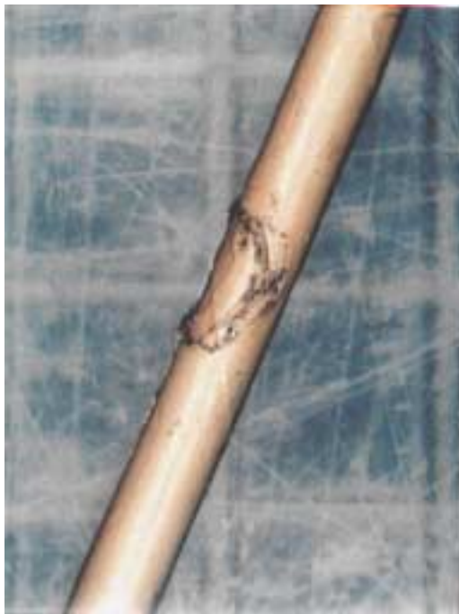
Figure 4-23: L-1011, LCL-L (polyimide) blister along wire.
