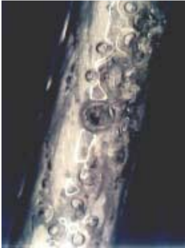
Figure 4-19: DC-9-2, CDT-E (Nylon/Glass/PVC) bubbles in outer insulation
