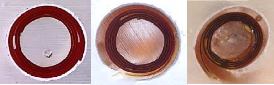
Figure 4-4: Cross section of A300 wires (FEP, polyimide) with conductor removed, from a typical section (left), and the atypical LCL Midspan (middle, right).
