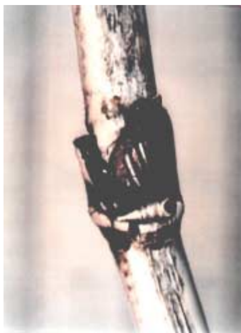
Figure 4-14: 747, ENS-1 Zone 9 (alkene-imide), exposed conductor.
