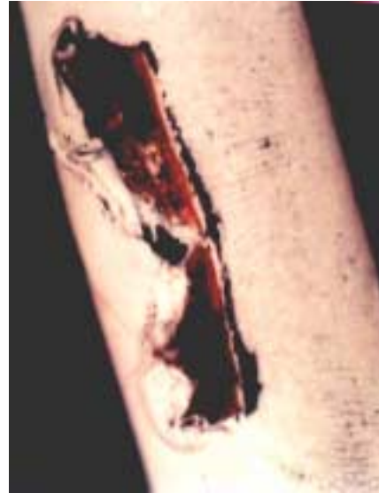
Figure 4-9: A-300, PSU-7 E, (FEP, polyimide) deep hot stamp marks along wire.
