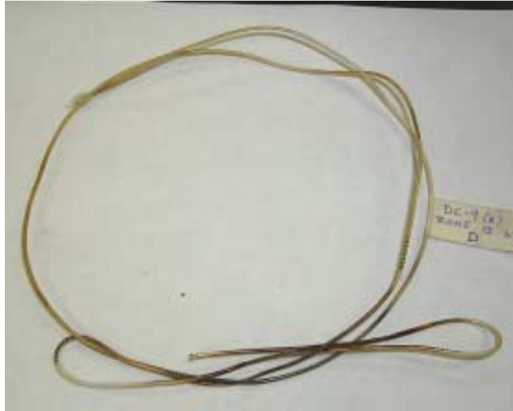
Figure 4-16: Wire from DC-9 (2) Zone 13 LWT (Nylon/Glass/PVC) that clearly demonstrates the range of conditions observed.
