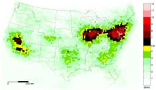
Figure 14. GPS Receiver Postcorrelation S/N_0 Degradation from DME/TACAN at 40,000 ft MSL over CONUS
