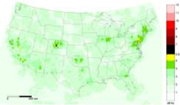
Figure 13. Total GPS Receiver Postcorrelation S/N_0 Degradation at 5,000 ft AGL over CONUS
