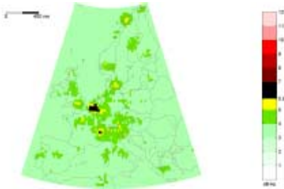
Figure 18. Total GPS Receiver Postcorrelation S/N_0 Degradation at 5,000 ft AGL over Europe
