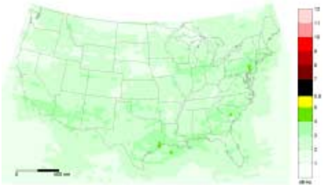
Figure 15. Total GPS Receiver Postcorrelation S/N_0 Degradation at 40,000 ft MSL over CONUS, DME/TACAN Emitters at 1176.45 \pm 10 MHz Reassigned
