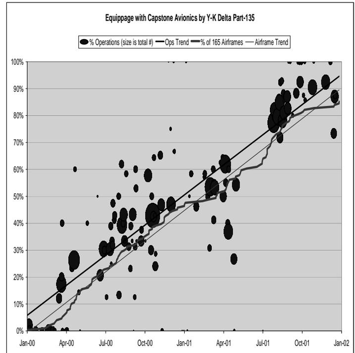
**Figure 3 YK Delta-based Part-135 Equipage with Capstone Avionics: Percentage of Arrivals and Departures during SVFR at Bethel and Percentage of the 165 active Airframes**
