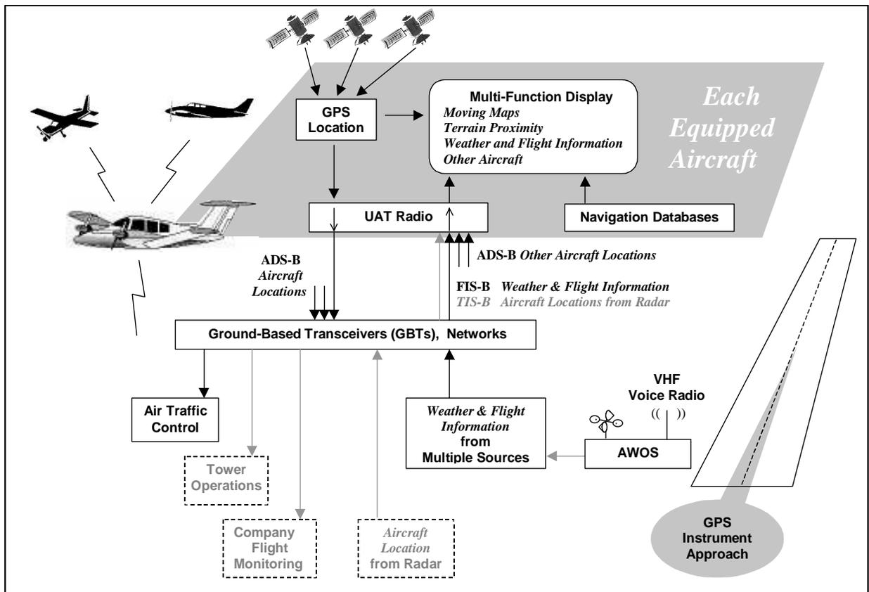
**Figure 2. Capstone Avionics, Ground Systems, and Capabilities**
